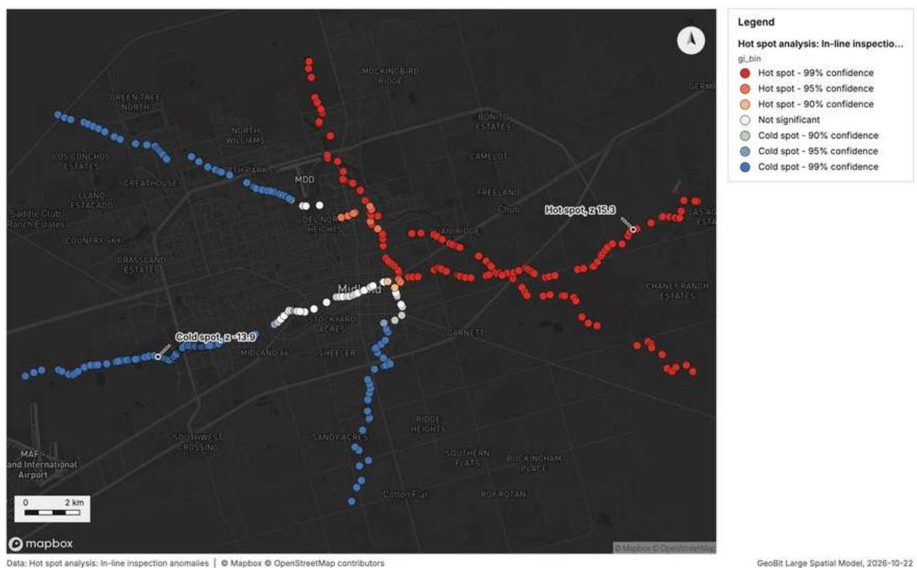
Figure 5. Hot spot analysis: In-line inspection anomalies [50]
