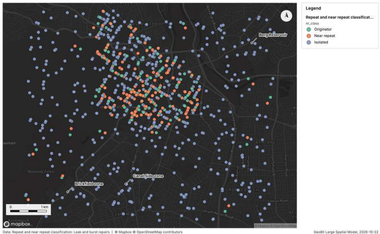
Figure 21. Repeat and near repeat classification: Leak and burst repairs [68]
